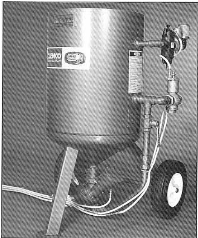
Sentinel Pneumatic Remote Control System with TLR-300
